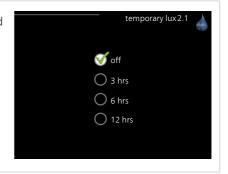
When hot water requirement has temporarily increased this menu can be used to select an increase in the hot water temperature to lux mode for a selectable time.
