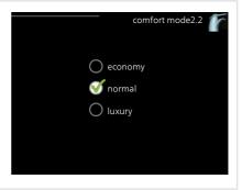
The difference between the selectable modes is the temperature of the hot tap water. Higher temperature means that the hot water lasts longer.
