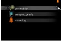
alarm log displays the latest alarm and information about the heat pump when the alarm occurred.
