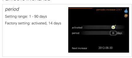
To prevent bacterial growth in the water heater, the heat pump can increase the hot water temperature for a short time at regular intervals.
