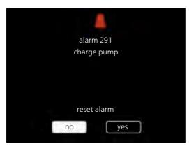
In the event of an alarm, a malfunction has occurred, which is indicated by an alarm symbol in the display.
