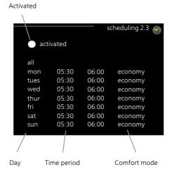
Day: Select which day or days of the week the scheduling is to apply to here. To remove the scheduling for a particular day, the time for that day must be reset by setting the start time to the same as the stop time. If the row "all" is used, all days in the period are set according to that row.
