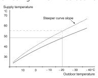
The optimum slope depends on the climate conditions in your location, if the house has radiators or under floor heating and how well insulated the house is.
