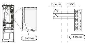
The example above uses the inputs AUX1 (X6:9-10) and AUX2 (X6:11-12) on the input circuit board (AA3).
