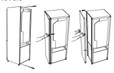
The side covers can be removed to facilitate the installation.
