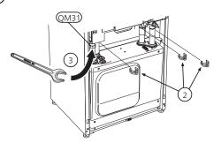
Disconnect the pipe connection at the shut-off valve (QM31).
