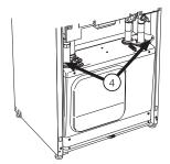
Remove the connection from the base card (AA2) using a screwdriver.
