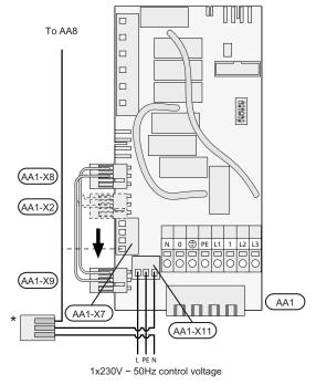
\* Only with separate earth-fault breaker.
