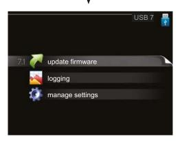
When a USB memory is connected a new menu (menu 7) appears in the display.
